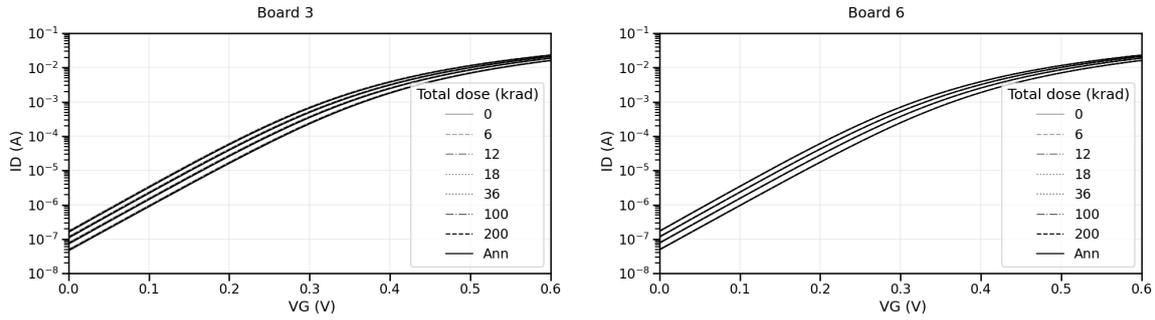
Figure 19: Characteristic curves for the NMOS2 transistor. Results for board 3 (left) compared to board 6 (right).
