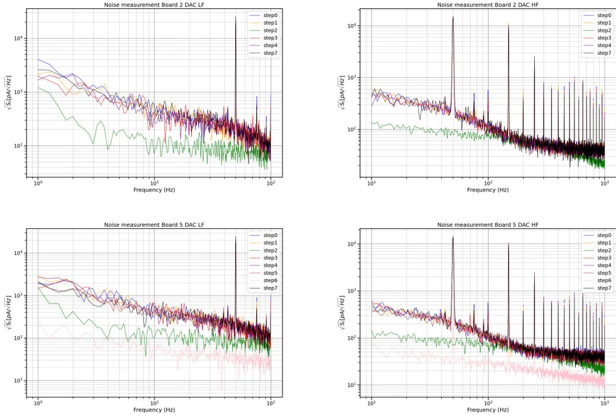
Figure 26: Current noise density ( $\sqrt{S_I}$ ) for the DAC of boards 2 and 5 in the low frequency (left) and high frequency (right) ranges.
