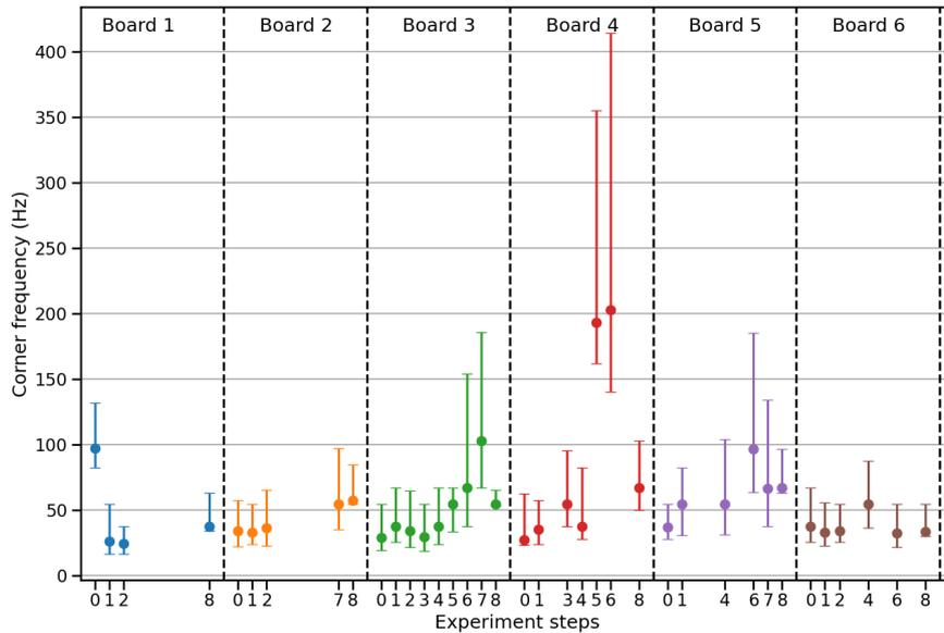
Figure 31: Corner frequencies for all the boards found applying the finding method. Error bar plot are used to visualize the data presented in Table 8. Bullet symbols represent the mean white noise value, while the upper and lower sticks represent the error of the finding method.
