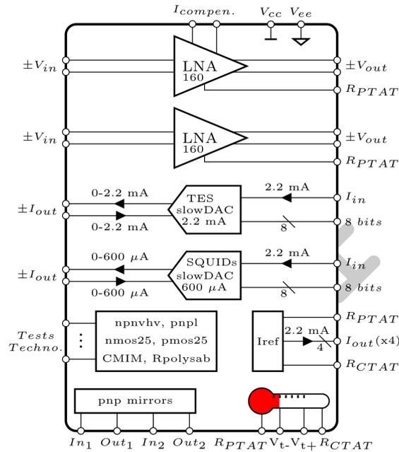
Figure 3: Block diagram of the AwaXe\_v4 ASIC including all internal devices.
