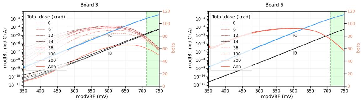
Figure 14: Gummel plots of the PNP device in the ASIC. Results for board 3 (left) compared to board 6 (right).
