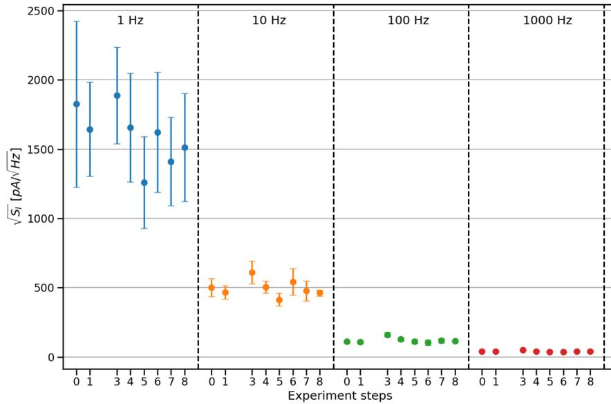
Figure 32: Evolution of the DAC noise over frequency in all the measurement steps.
