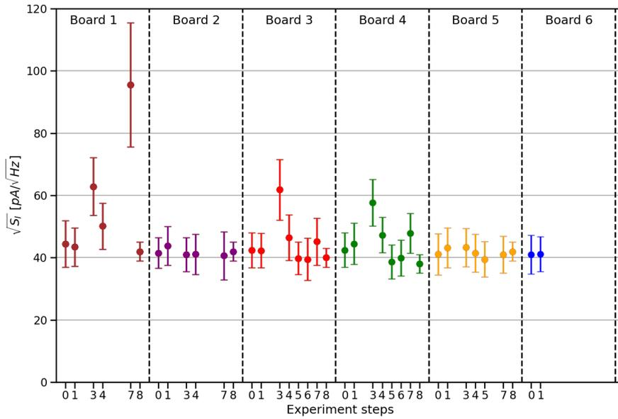
Figure 28: Current noise density of the DACs in the analyzed white noise region (300 – 1000 Hz).
