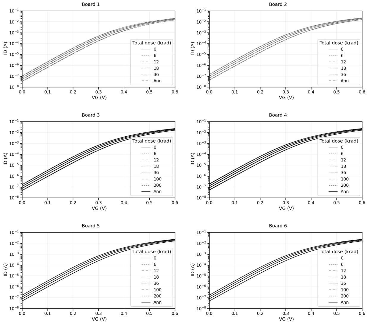
Figure 45:  $I_d$  vs  $V_{gs}$  plot for the PMOS device in the 6 boards.
