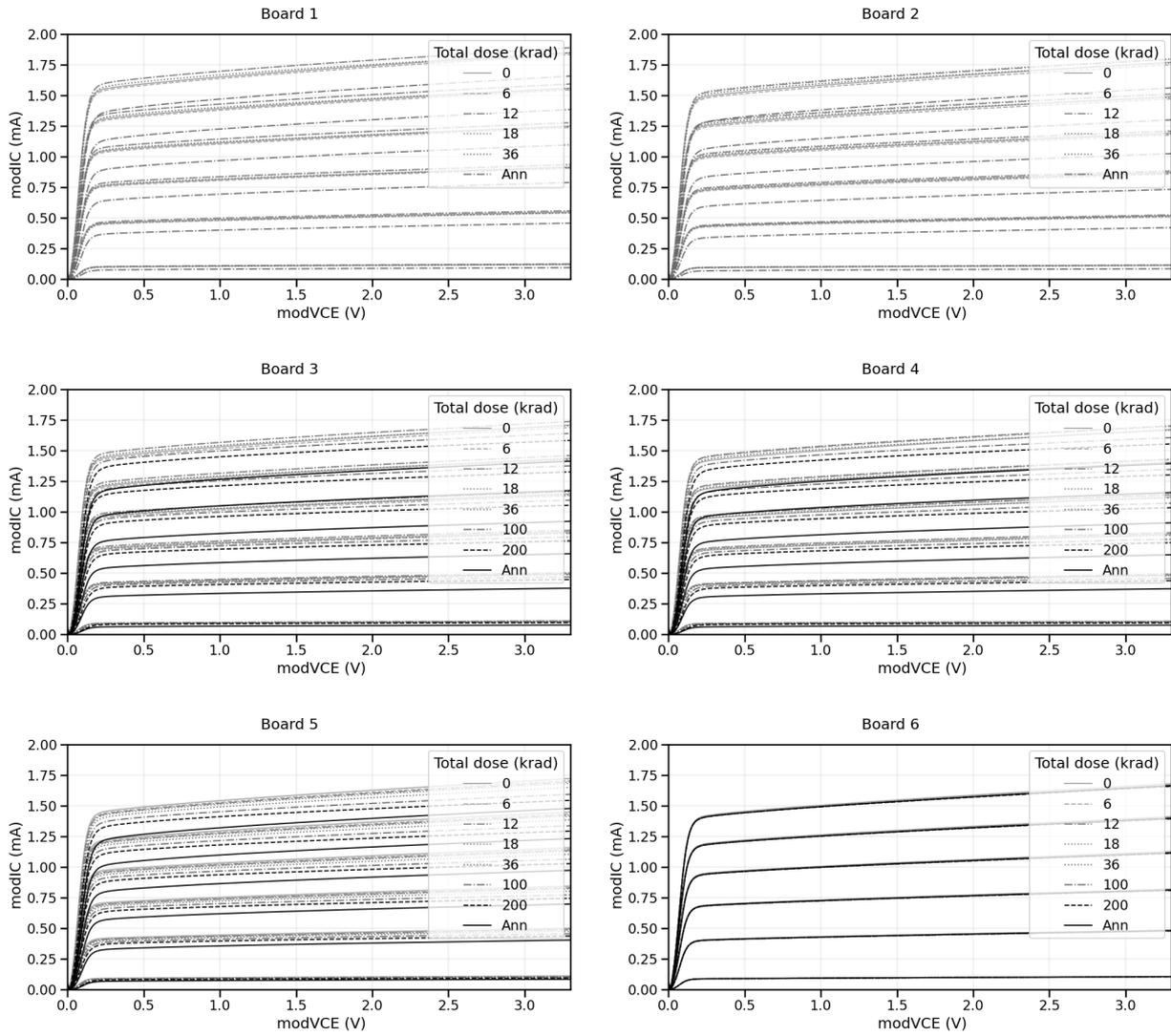
Figure 40:  $I_b$  and  $I_c$  vs  $V_{ce}$  plot for the PNP device in the 6 boards.
