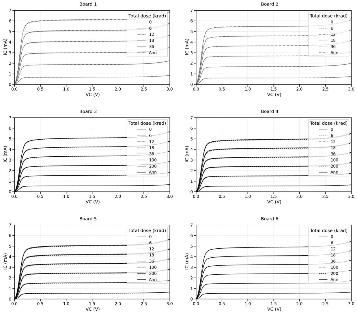
Figure 38:  $I_b$  and  $I_c$  vs  $V_{ce}$  plot for the NPN2 device in the 6 boards.
