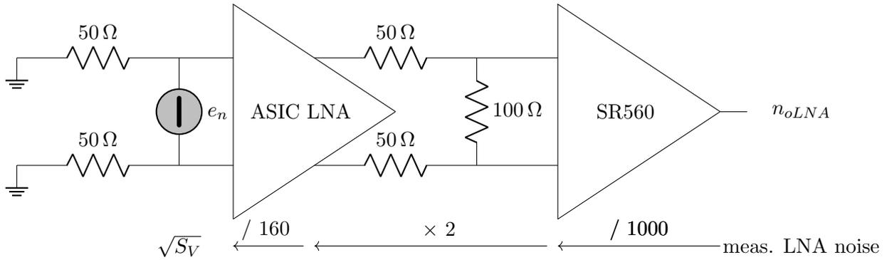
Figure 24: Electronic schematic showing the LNA noise measurement setup.
