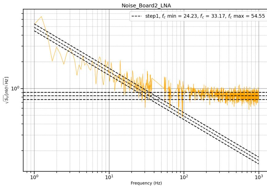
Figure 30: Corner frequency finding method applied to the board 2 in *step 1*.
