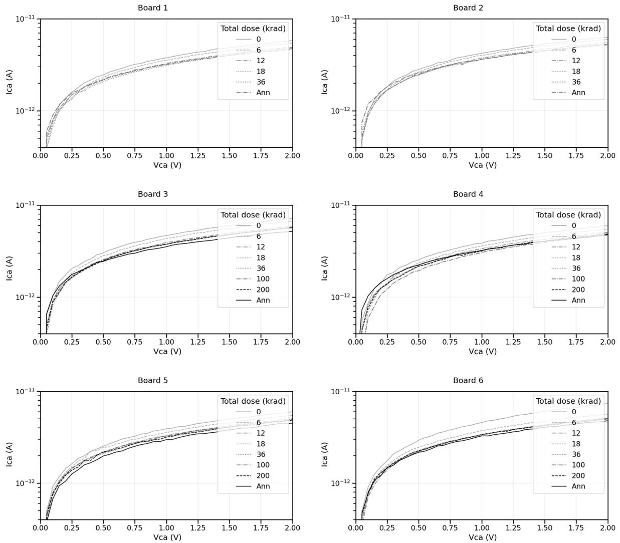
Figure 47: C leakage in the 6 boards.
