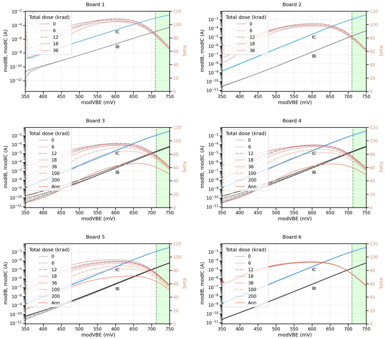
Figure 39: Gummel plot for the PNP device in the 6 boards.
