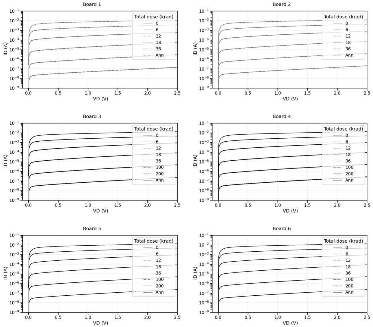
Figure 44:  $I_d$  vs  $V_{ds}$  plot for the NMOS2 device in the 6 boards.
