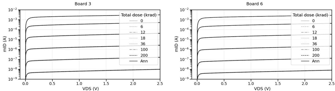
Figure 22: Characteristic curves for the PMOS transistor. Results for board 3 (left) compared to board 6 (right).
