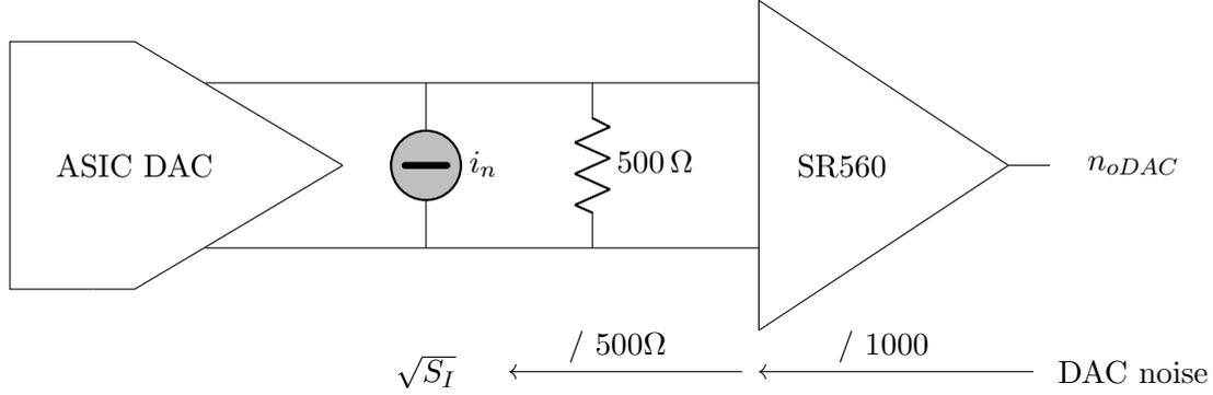
Figure 25: Electronic schematic showing the DAC noise measurement setup.
