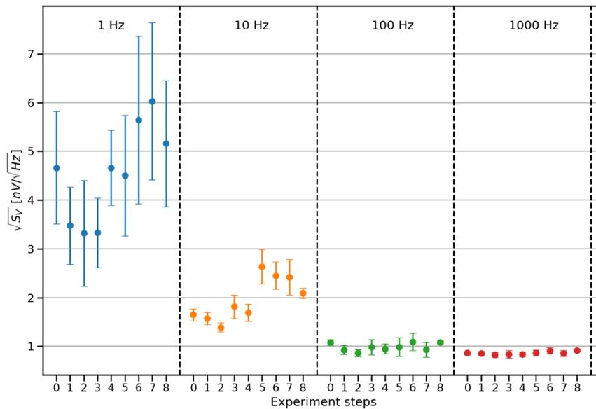
Figure 33: Evolution of the LNA noise over frequency in all the measurement steps.
