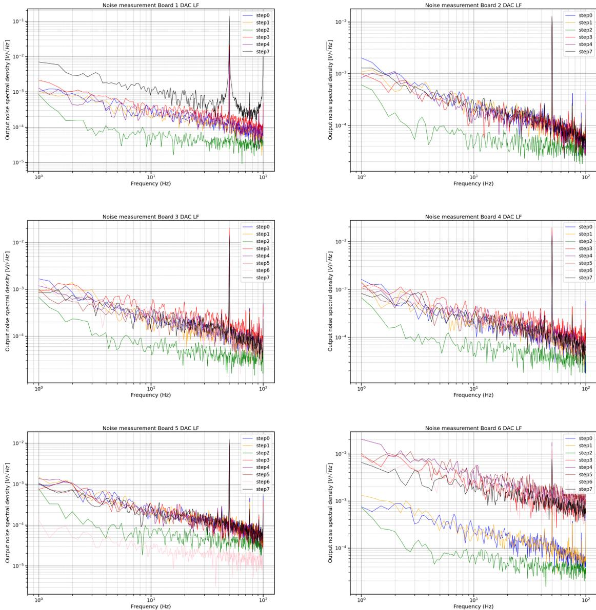
Figure 48: Output noise of the DAC measurements in the frequency range from 1 Hz to 100 Hz. Raw data, not taking into account the gains/losses in the measurement setup.
