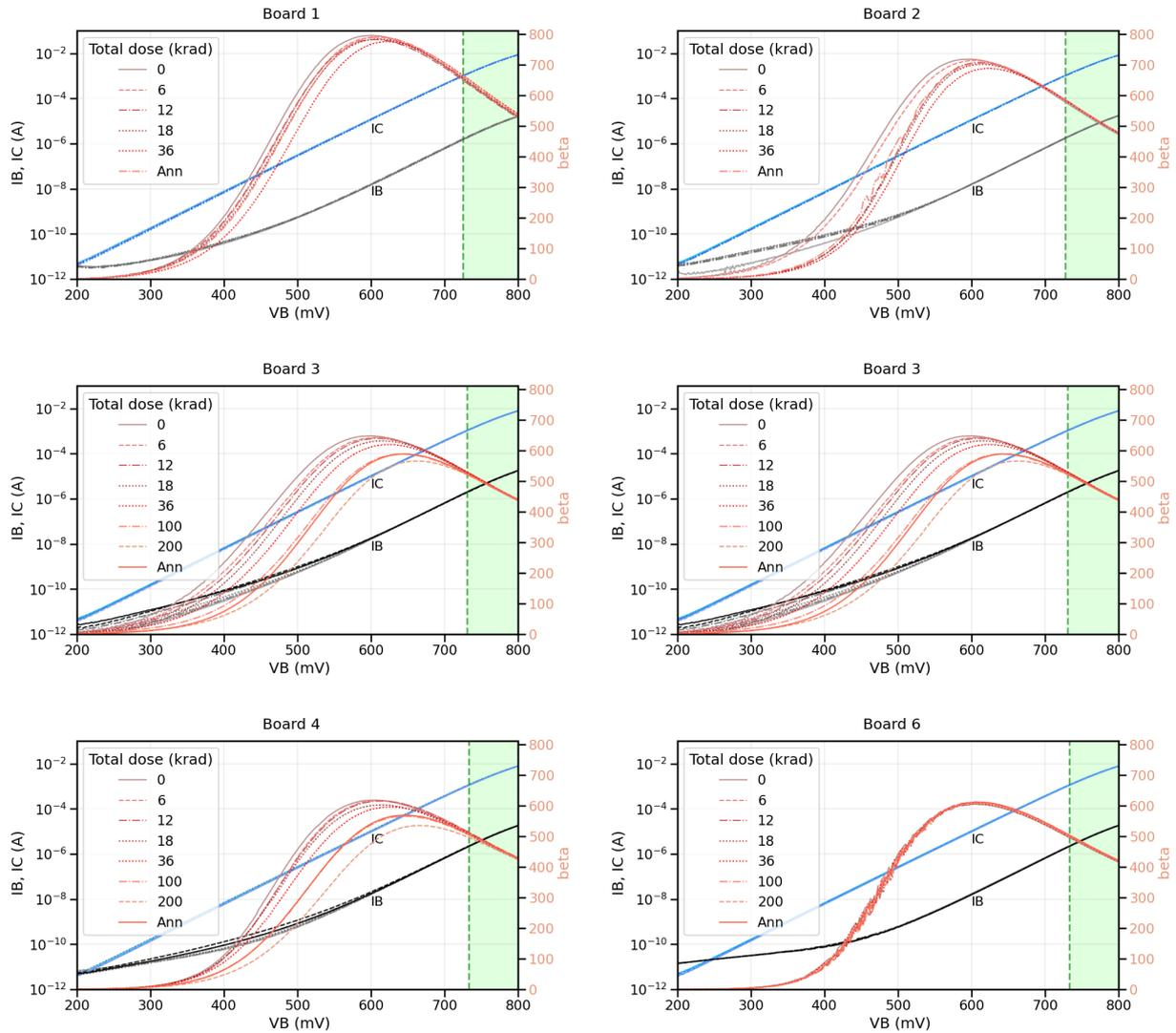
Figure 35: Gummel plot for the NPN1 device in the 6 boards.
