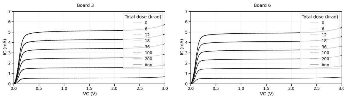
Figure 11: Characteristic curve of the NPN1 transistor. Results for board 3 (left) compared to board 6 (right).
