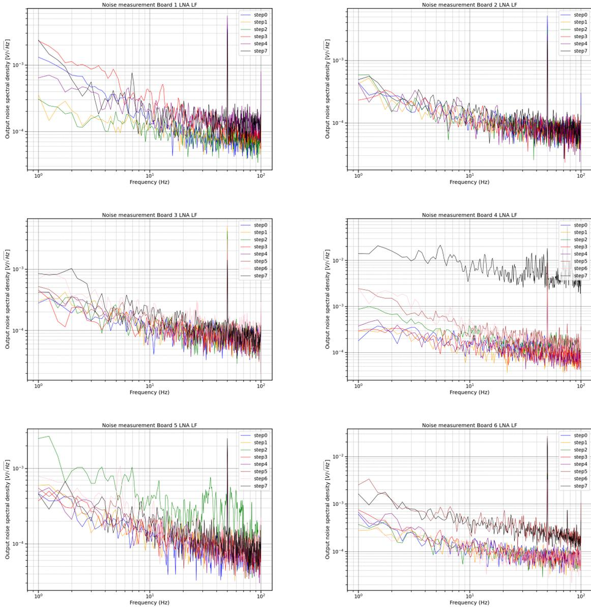
Figure 50: Output noise of the LNA measurements in the frequency range from 1 Hz to 100 Hz. Raw data, not taking into account the gains/losses in the measurement setup.
