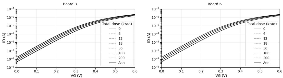
Figure 17: Characteristic curves for the NMOS1 transistor. Results for board 3 (left) compared to board 6 (right).
