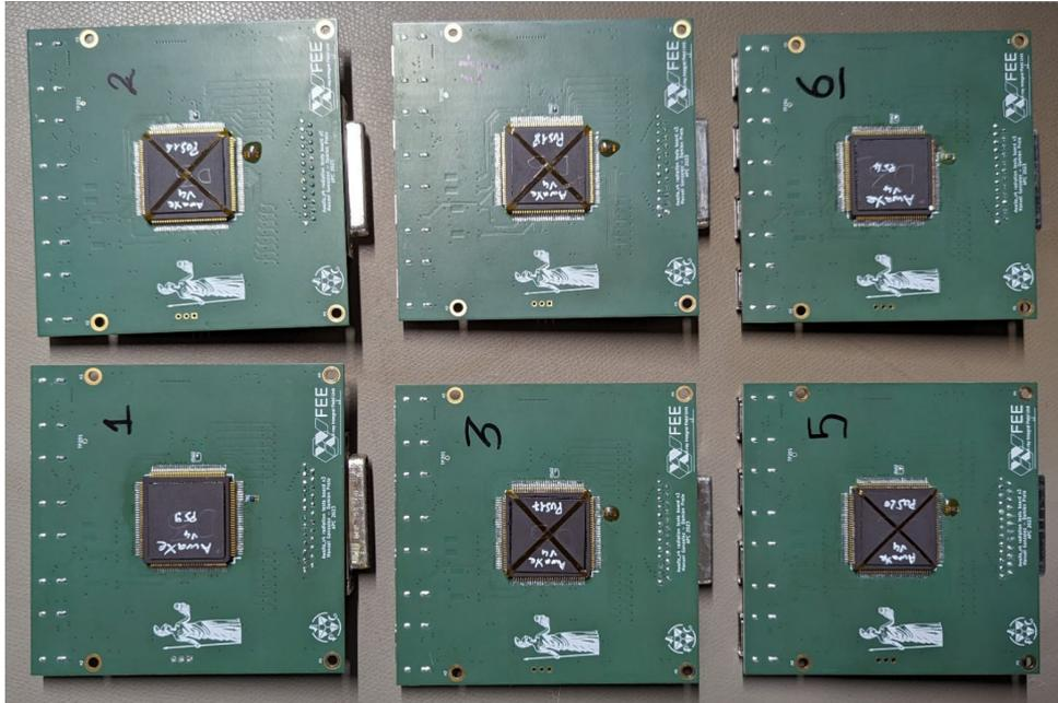
Figure 1: The ASIC boards used in the TID tests
