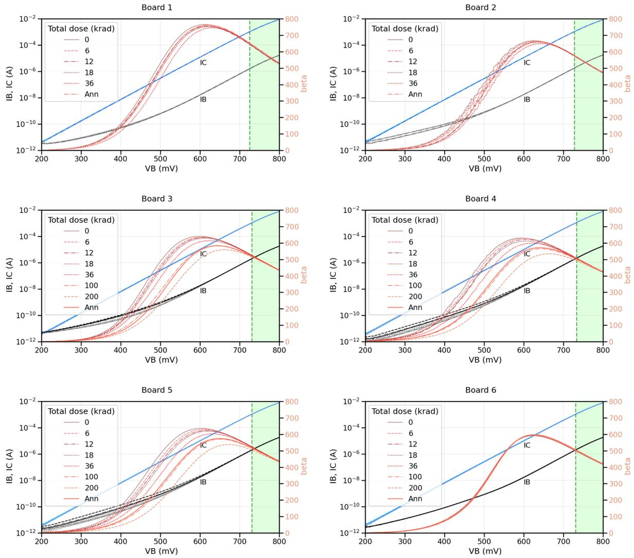
Figure 37: Gummel plot for the NPN2 device in the 6 boards.
