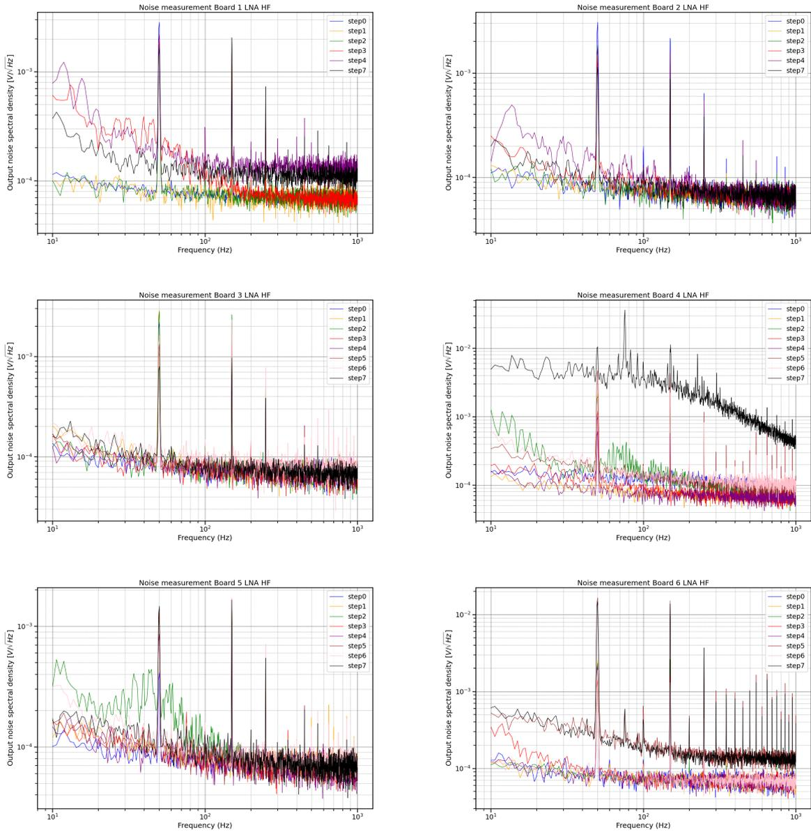
Figure 51: Output noise of the LNA measurements in the frequency range from 10 Hz to 1000 Hz. Raw data, not taking into account the gains/losses in the measurement setup.
