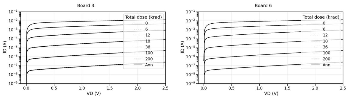
Figure 18: Characteristic curves for the NMOS1 transistor. Results for board 3 (left) compared to board 6 (right).
