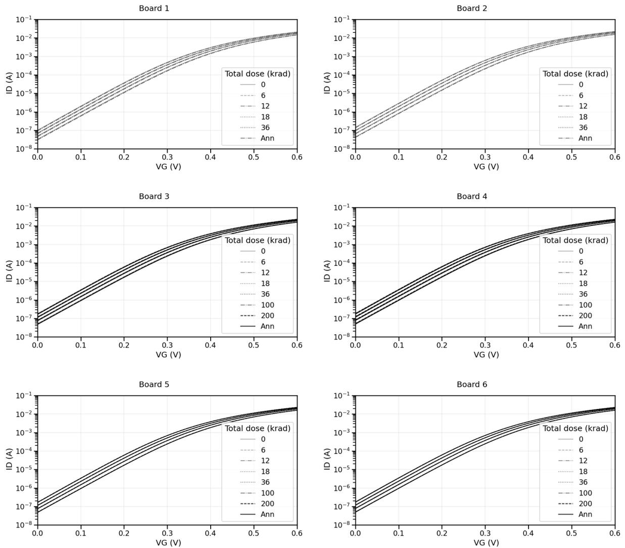
Figure 41:  $I_d$  vs  $V_{gs}$  plot for the NMOS1 device in the 6 boards.
