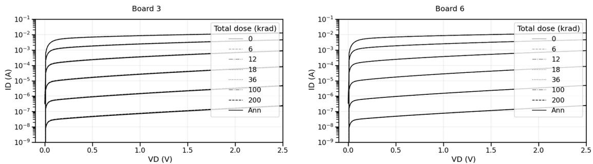
Figure 20: Characteristic curves for the NMOS2 transistor. Results for board 3 (left) compared to board 6 (right).
