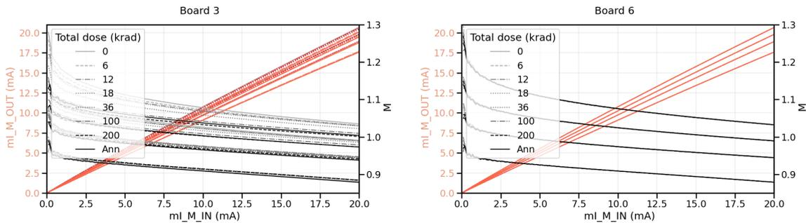
Figure 9: Characterization of the PNP current mirror. Results of board 3 (left) compared to the results of the characterization of board 6 as a reference (right).
