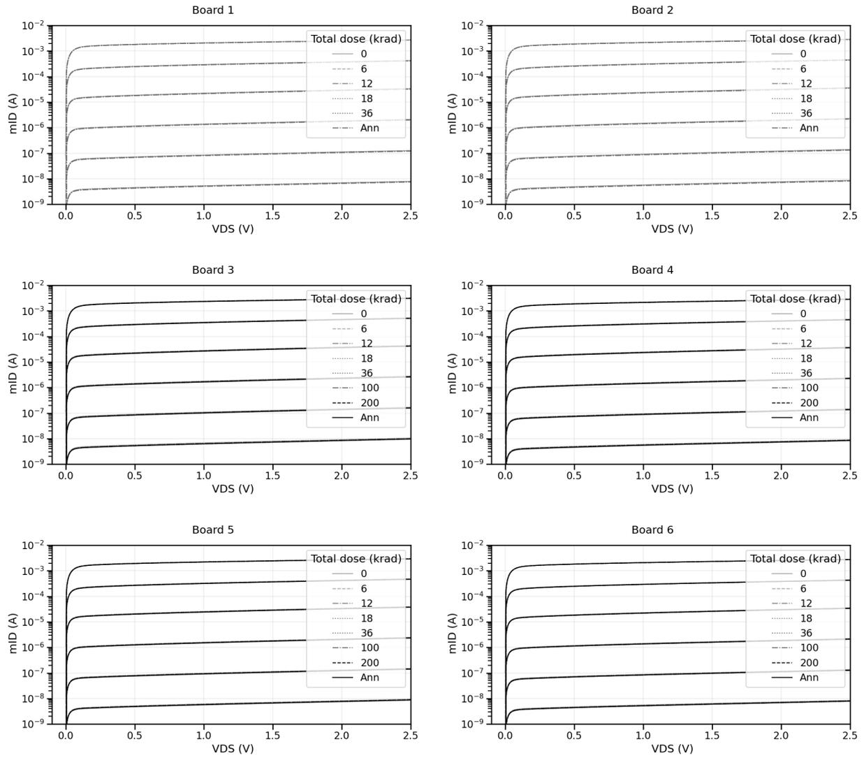
Figure 46:  $I_d$  vs  $V_{ds}$  plot for the NMOS2 device in the 6 boards.
