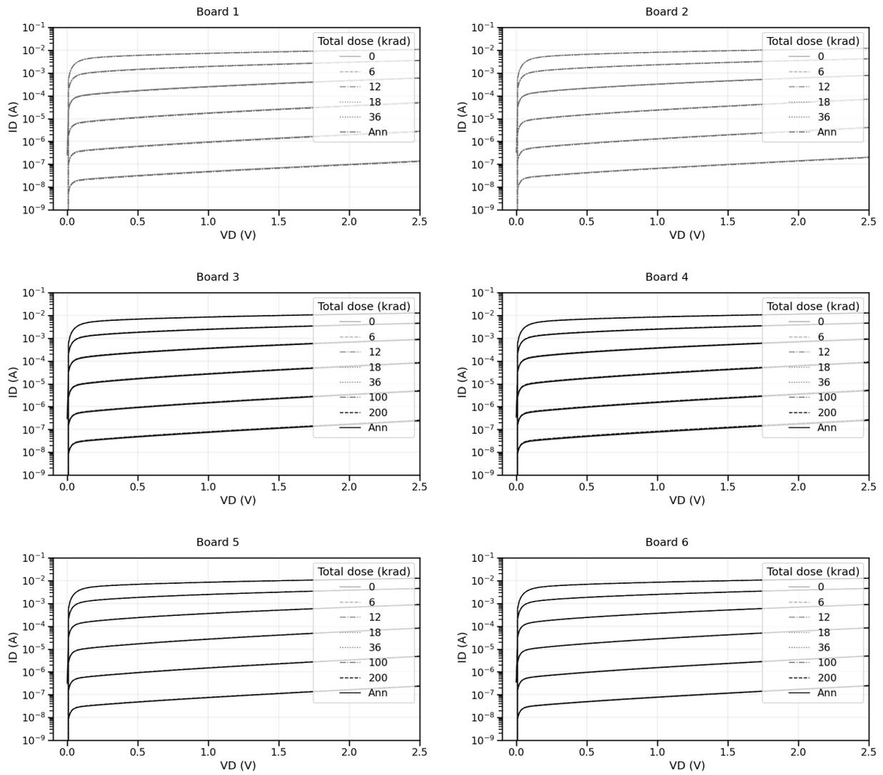
Figure 42:  $I_d$  vs  $V_{ds}$  plot for the NMOS1 device in the 6 boards.
