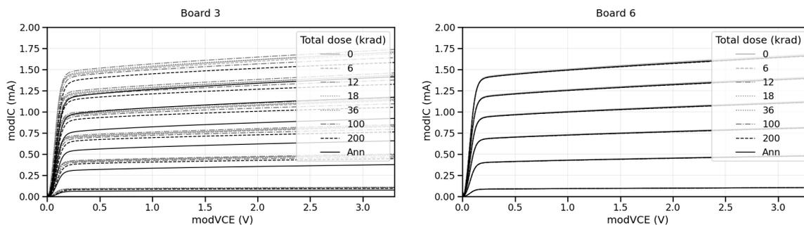
Figure 15: Characteristic curve of the PNP transistor. Results for board 3 (left) compared to board 6 (right).
