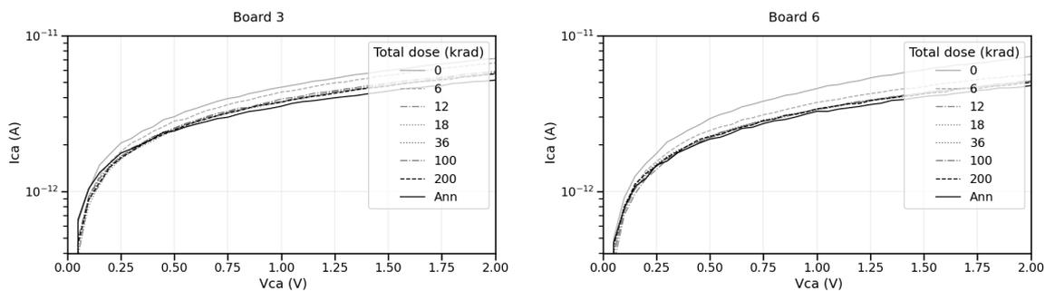
Figure 23: Leakage current due to in-chip MIM capacitor. Results for board 3 (left) compared to board 6 (right).
