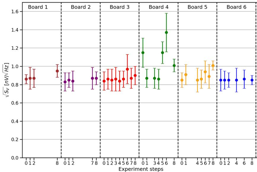
Figure 29: Voltage noise density of the LNAs in the analyzed white noise region (300 – 1000 Hz).
