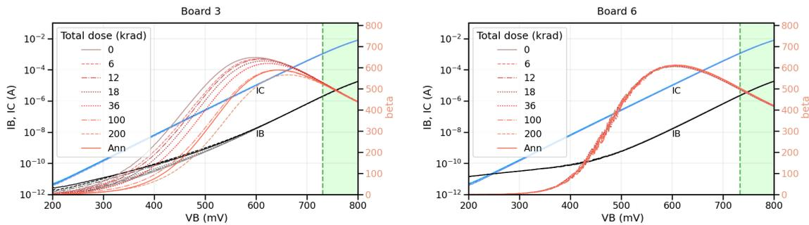
Figure 10: Gummel plots of the NPN1 device in the ASIC. Results for board 3 (left) compared to board 6 (right).
