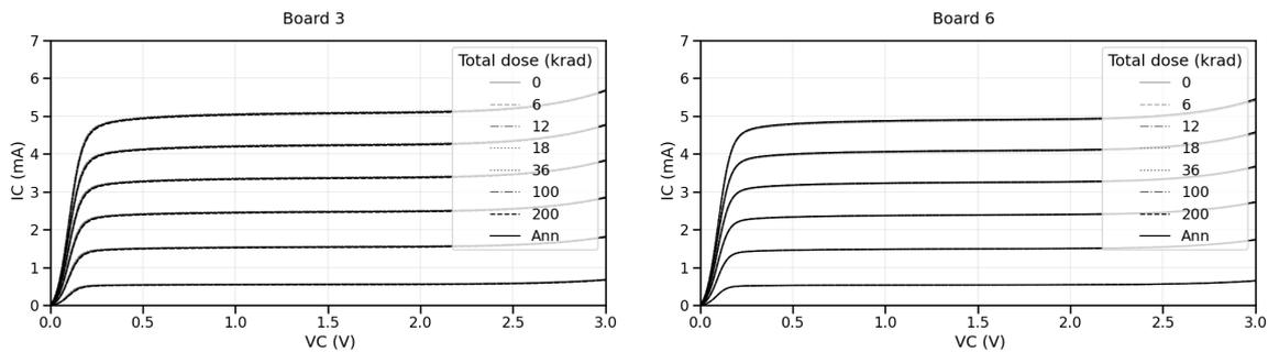
Figure 13: Characteristic curve of the NPN2 transistor. Results for board 3 (left) compared to board 6 (right).
