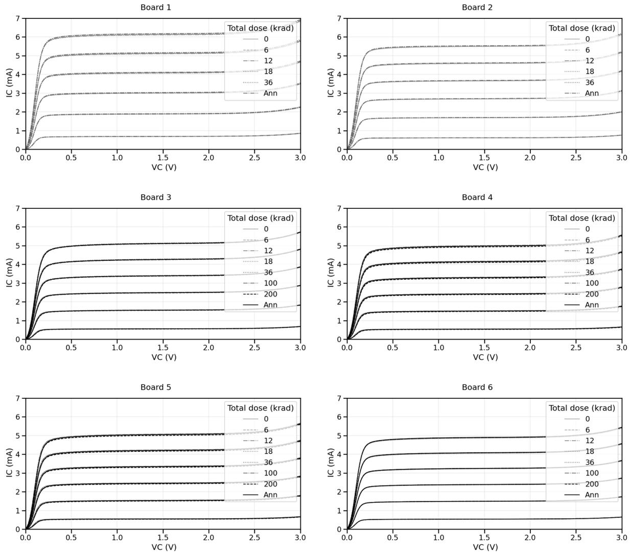
Figure 36:  $I_b$  and  $I_c$  vs  $V_{ce}$  plot for the NPN1 device in the 6 boards.
