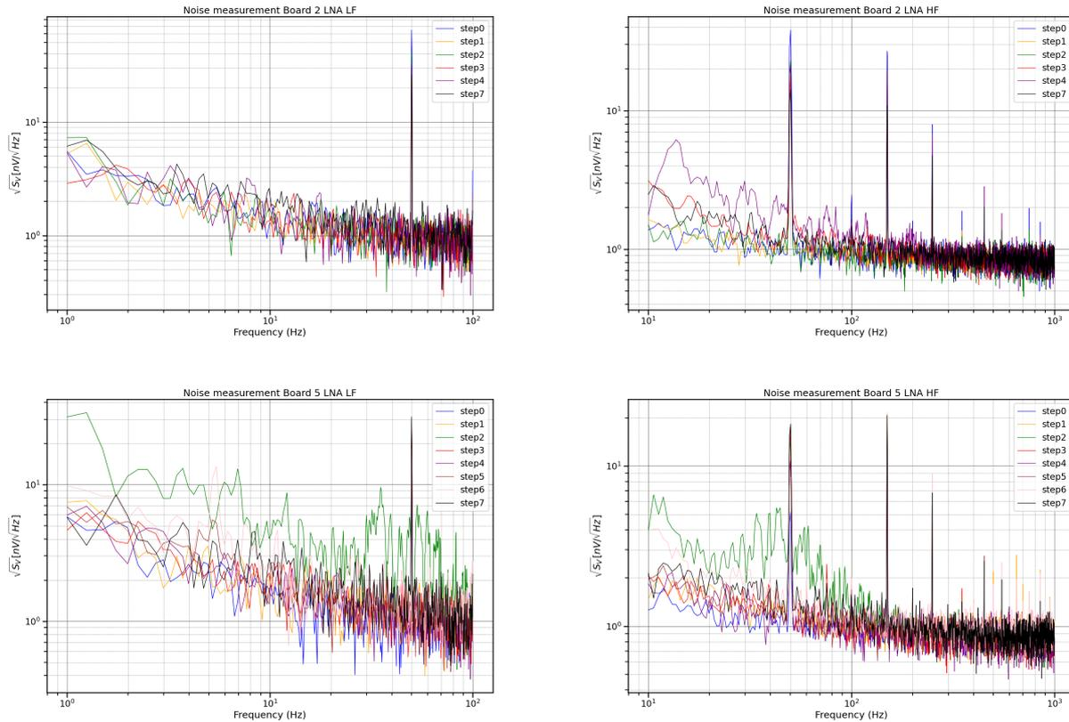
Figure 27: Voltage noise density ( $\sqrt{S_V}$ ) for the LNA of boards 2 and 5 in the low frequency (left) and high frequency (right) ranges.
