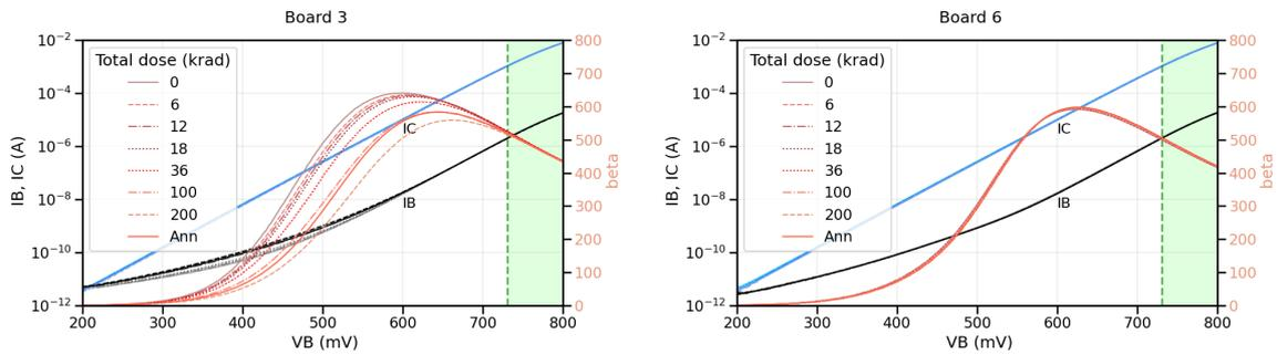
Figure 12: Gummel plots of the NPN2 device in the ASIC. Results from board 3 (left) compared to board 6 (right).
