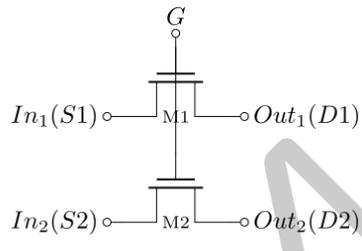
Figure 16: Simplified schematic of the NMOS switches present in the AwaXe\_v4 ASIC.
