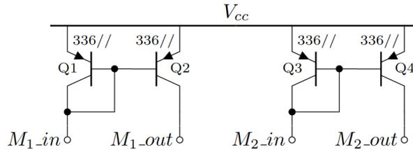
Figure 8: Two PNP current mirrors within the ASIC.
